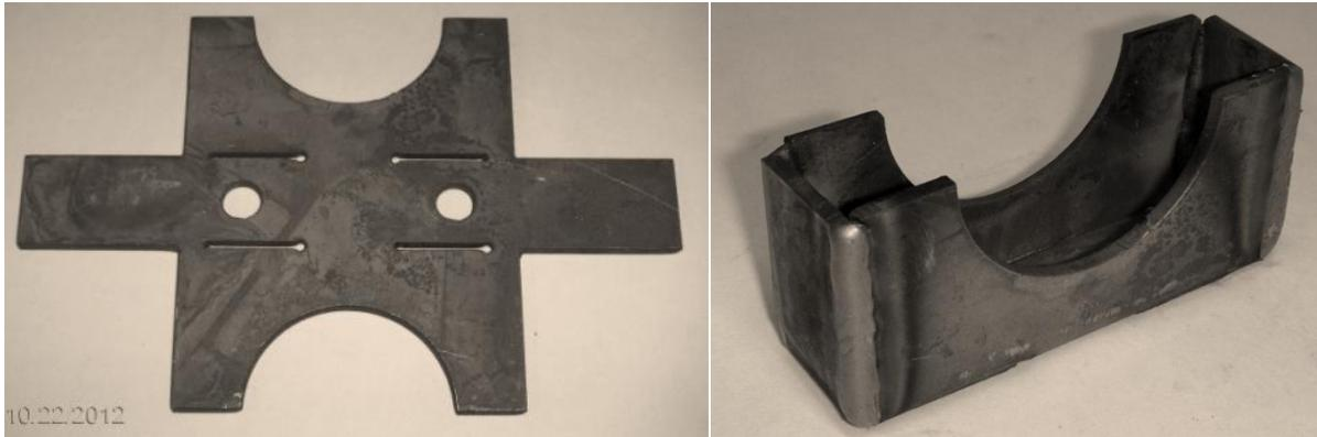
Fold all 4 sides of the pattern holder bracket upwards and weld as shown.
