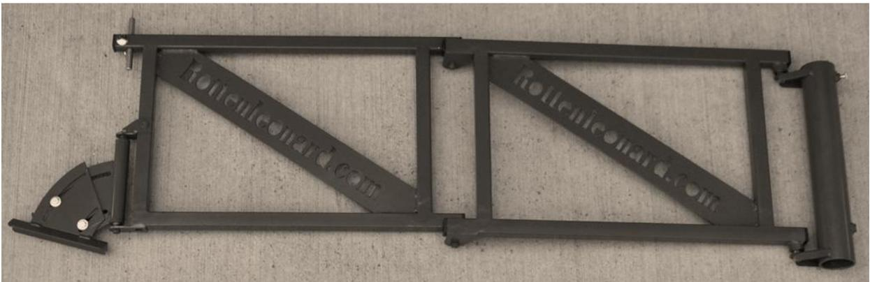
The assembly can now be mounted to any 2" O.D. tube mounted to your welding table. We recommend that the stand pipe be adjustable to allow the tracer to be squared up to your table as needed. Also constructing adjustable height "feet" to place under your material is very handy for quick and precise adjustments. You can find a video of the tracer in action at [www.rottenleonard.com](http://www.rottenleonard.com)
