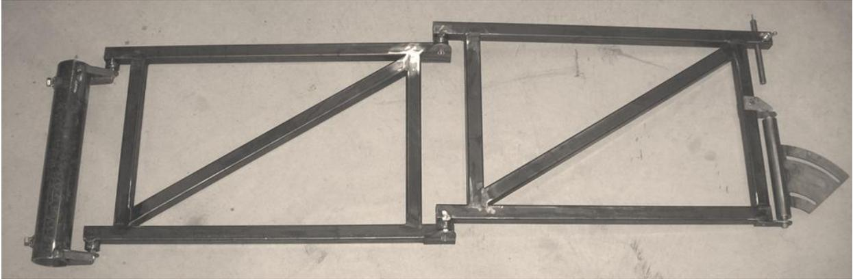
Using an appropriate size socket and hammer drive the bearings into the bearing cups, and assemble the tracer as shown in the above image.
