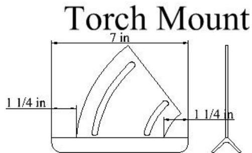
The torch mount is made from a 7" length of 1" angle iron, round the corners as shown in the drawing, then weld the bracket vertically and centered on the corner of the angle iron as shown. The torch can be mounted using hose clamps or similar devises.
