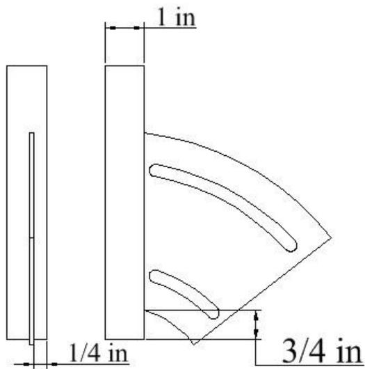
The Torch mount pivot bracket needs to be welded off center to allow the torch mount bracket to be centered on the pivot point when bolted on the left side of the pivot bracket, This can easily be accomplished by laying the tube on a flat surface, followed by laying the pivot bracket on top of a 1/4" piece of flat stock. Be sure to position the bracket 3/4" from the bottom of the pivot tube.
