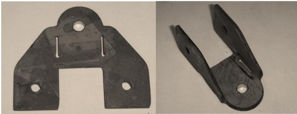
Finish drill the Plasma Torch adapter upper mount Clamp holes to 1/4", then clamp and fold the mount around a length of 1" square tube as shown above.
