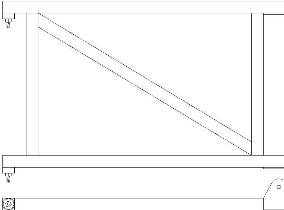
Weld on the bearing cups as shown in the image making sure the machined inner surface is pointed away from the frame. Also weld on the tracer hinge brackets and finish drill the bolt hole to 5/16".
