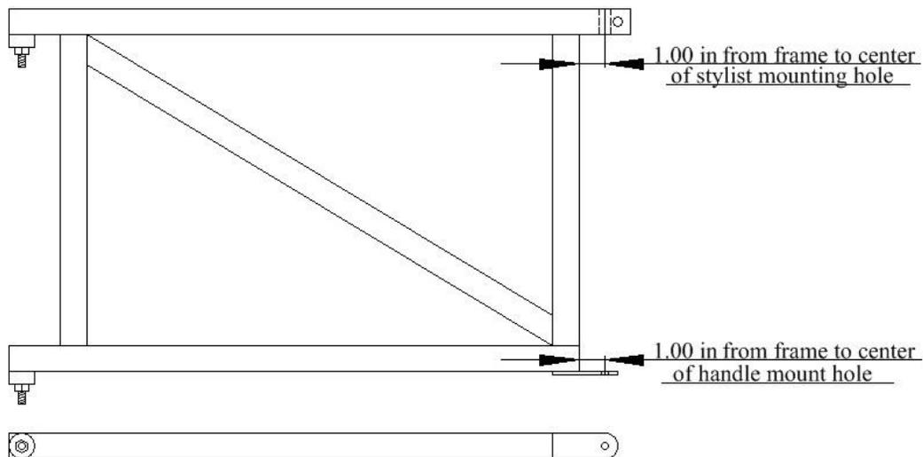
Weld on the bearing cups as shown in the image making sure the machined inner surface is pointed away from the frame. Also weld on the torch handle lower bracket and finish drill the bolt hole to 1/4".
