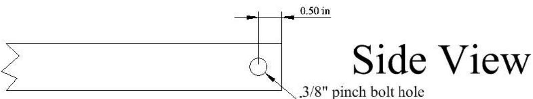
Modify a 24" length of 1" square tubing as shown in the diagram above to serve as a stylus holder. You may use a small file to make one of the pinch bolt holes square to accept a carriage bolt, otherwise you can insert a 3/8" x 1 1/2" bolt and tack weld.
