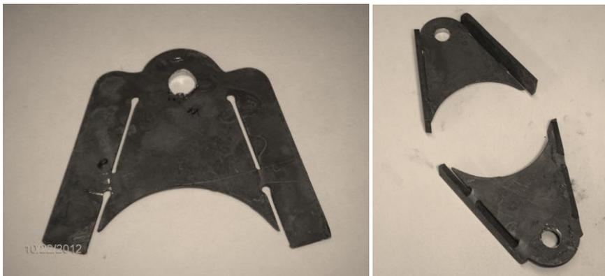
Finish drill the tracer frame mounting brackets holes to 5/16" then fold both as shown.
